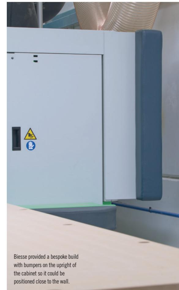
Biesse provided a bespoke build with bumpers on the upright of the cabinet so it could be positioned close to the wall.
