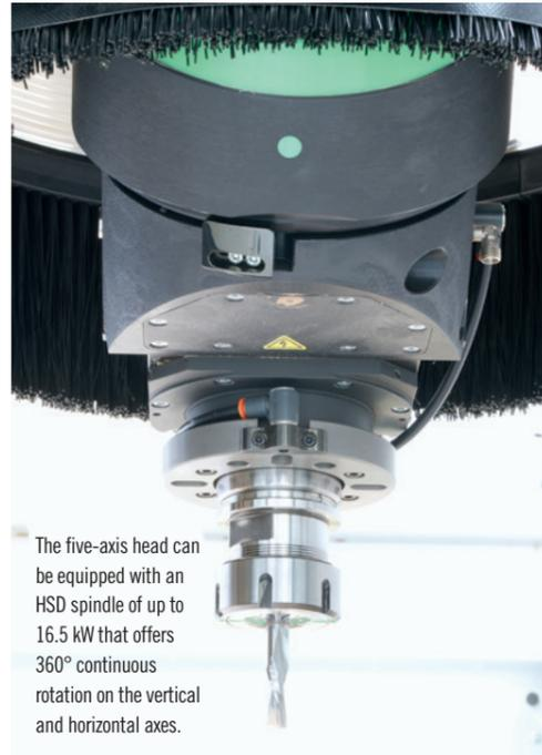
The five-axis head can be equipped with an HSD spindle of up to 16.5 kW that offers 360° continuous rotation on the vertical and horizontal axes.
